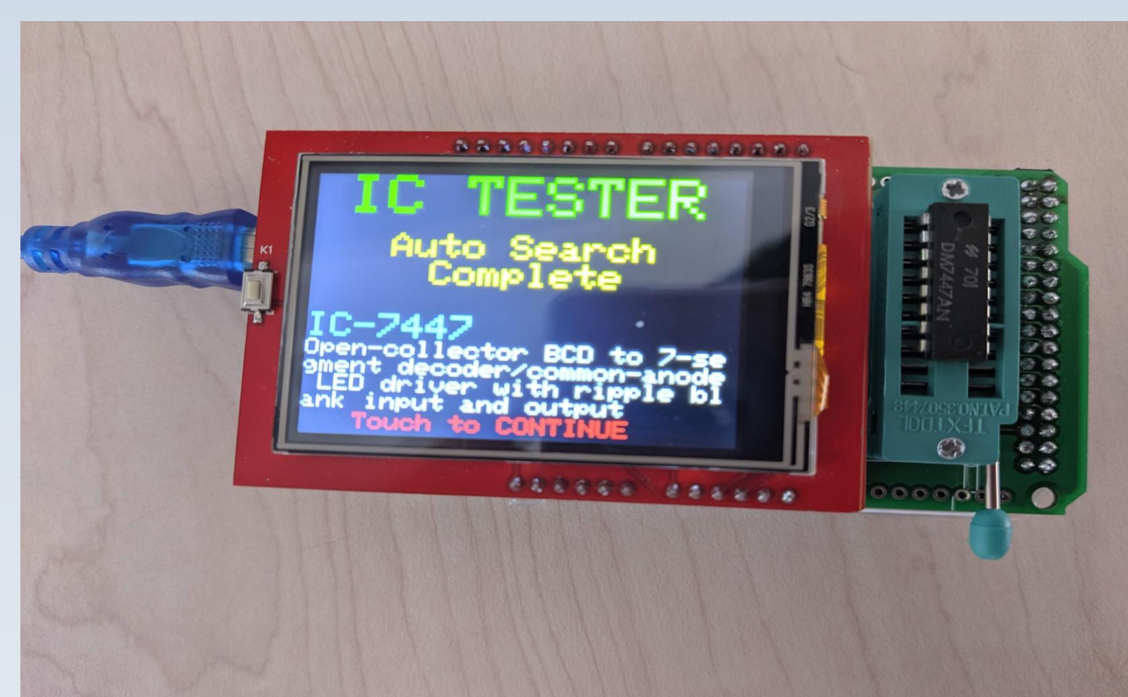
Fig. 3. The smart IC tester after performing a successful auto search. Note that the IC that is connected in the socket has the same number displayed in the screen.
