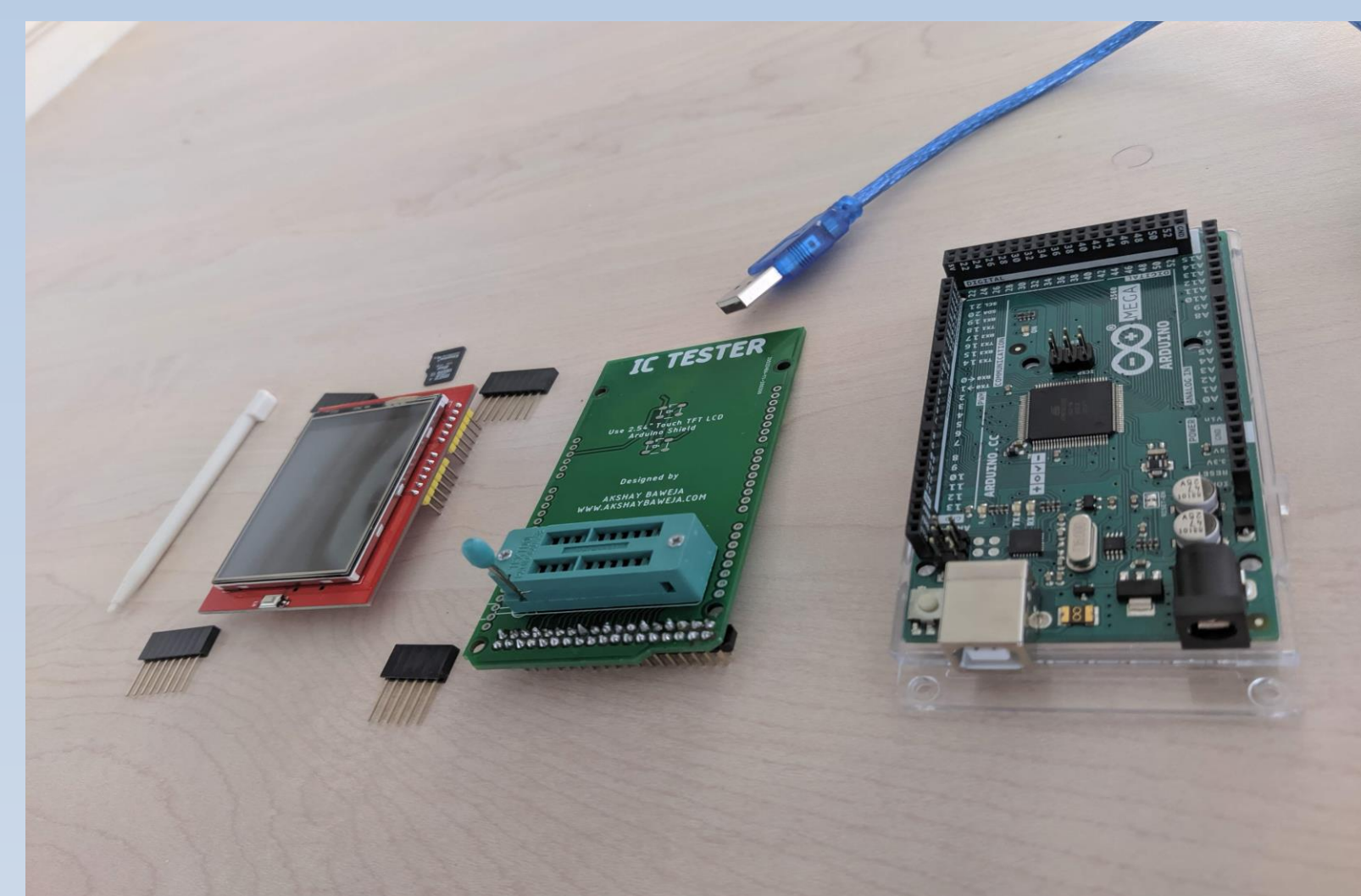
Fig. 1. Components needed to build the smart IC tester. From left to right: LCD touchscreen, PCB board with the socket already soldered, and the Arduino Mega board.
