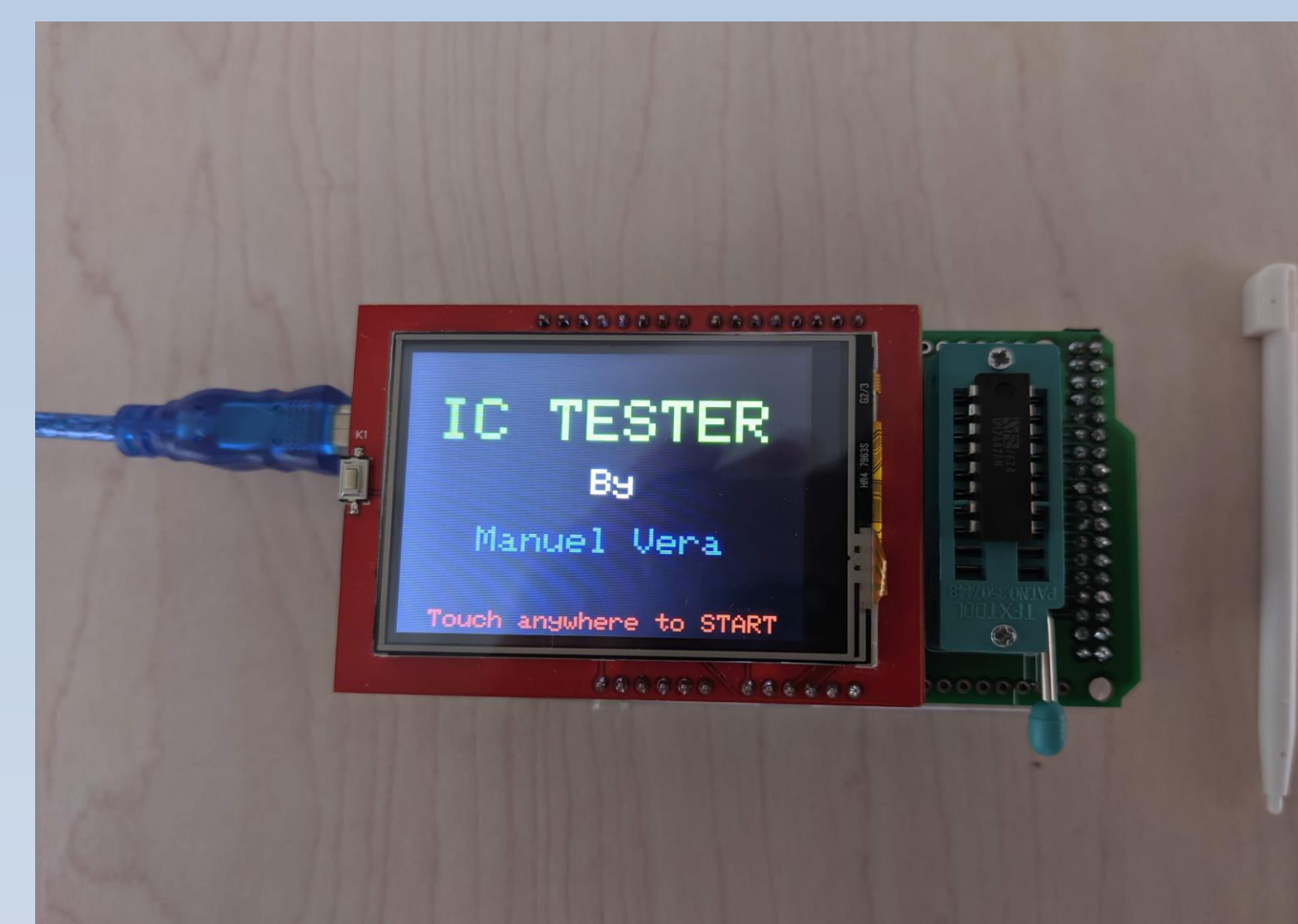
Fig. 2. The smart IC tester already assembled and turned on in the main menu screen.
