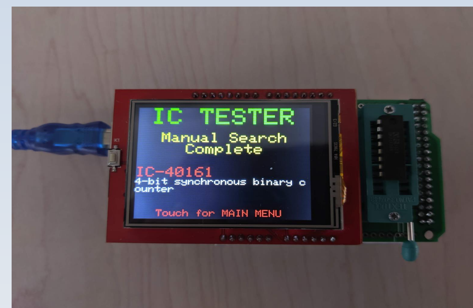
Fig. 4. The smart IC tester after completing a successful manual search. This type of search can be completed without connecting the IC into the socket.
